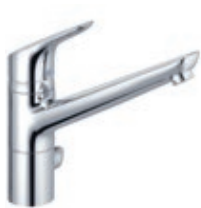
multi single lever sink mixer DN 15 swivelling spout (360°) connection for washing machine and dishwasher H1 210, H2 169, A 203, Ø2 52 325760575 ■
