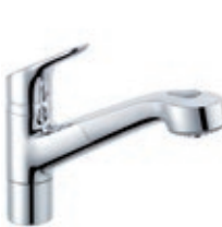
single lever sink mixer DN 15 with pull-out hand spray with diverter from shower to jet spray swivelling spout (110°) H1 204, H2 129, A 208, Ø1 34, Ø2 52 325810575 ■
