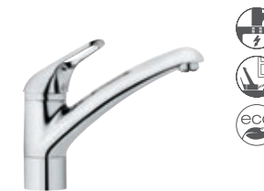
single lever sink mixer bayonette DN 10 for installation beneath windows swivelling spout (360°) for use with displacement heaters H1 185, H2 150, A 200, Ø1 35, Ø2 52 337930562 ■
